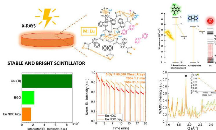
**Figure 1:** Structure of the Eu NDC bipy MOF and its energy levels. Results of RL intensity vs. commercial scintillators, RL stability under lab X-ray source, and structure stability (WAXs) under synchrotron radiation.
