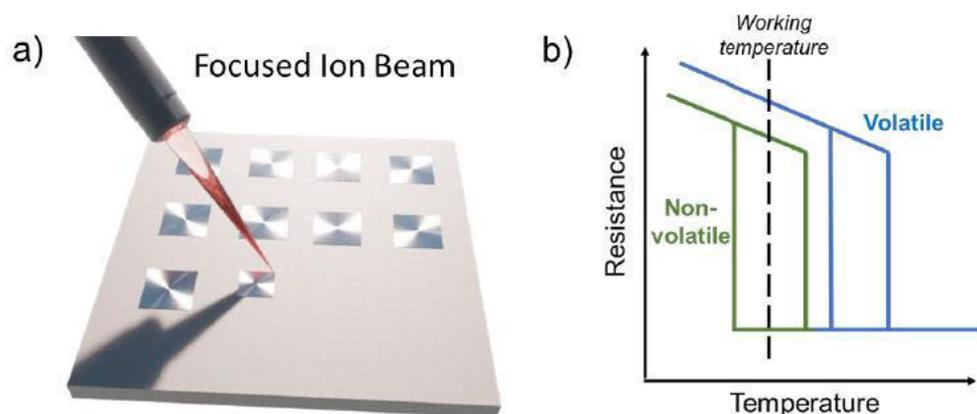
**Figure 1:** Key scheme for our single platform micrometric neural network based on VO<sub>2</sub>. a) FIB to locally tailor the MIT of VO<sub>2</sub> thin films. b) Representation of the hysteresis behavior of pristine (blue) and FIB radiated (green) zones, indicating the working temperature that will enable a volatile and nonvolatile transition for their implementation as neuristors and synaptors, respectively.
