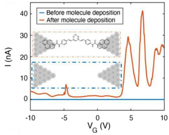
**Figure 1:** Current vs gate voltage before and after molecules deposition.
