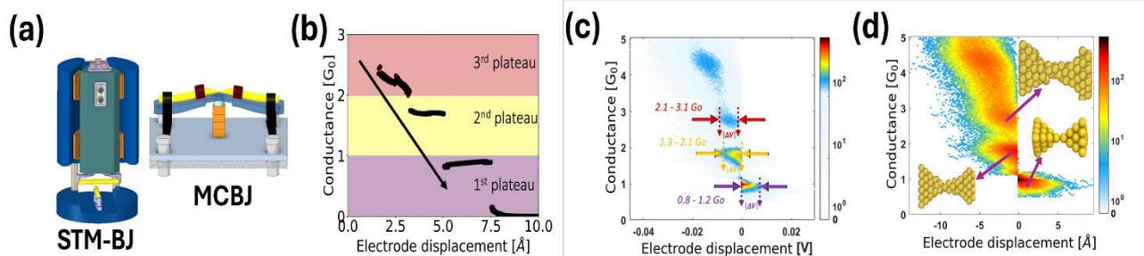
**Figure 1:** (a) shows an illustration of the STM and MCBJ experimental setups. (b) displays a rupture trace featuring three distinct plateaus. (c) presents a two-dimensional plot used for calibration. (d) shows a calibrated density plot of gold rupture traces, highlighting each structure.
