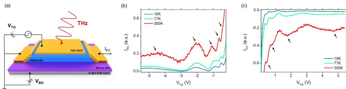
**Figure 1.** (a) Schematic 3D view of the zero-bias photocurrent measurements of the graphene plasmonic photodetector. Zero-bias normalized photocurrent for three selected temperatures of 10 K, 77K and 300K (room temperature) for negative (b) and positive (c) top gate potentials for an incident radiation of 2.5 THz. For easier visualization, the temperature dependence photocurrent shown in panels (b)-(c) are normalized with respect to the maximum near the charge neutrality point.
