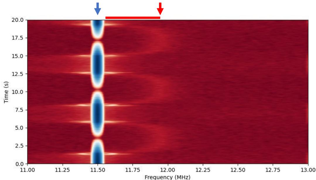
**Figure 1:** RF spectrum of reflected signal from a MoS<sub>2</sub> drum resonator illuminated with a 532 nm CW laser (2 mW) and driven by an amplitude-modulated 11.5 MHz RF signal. The electromechanical response is transduced as an amplitude modulation of the reflected signal at the actuation frequency (blue arrow). The optical response from the coupled optomechanical resonator (red arrow) is shifted towards the driving frequency as the amplitude increases.
