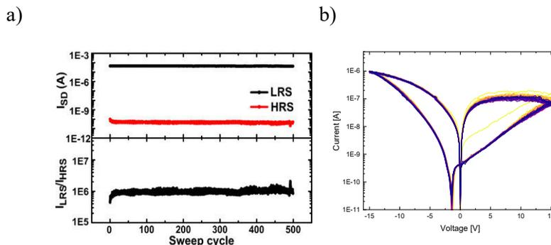
a) Endurance of high (HRS) and low (LRS) resistance states (top) and  $I_{LRS}/I_{HRS}$  at voltage bias of 7.5 V (bottom) of a 3-terminal MoS<sub>2</sub> device.
