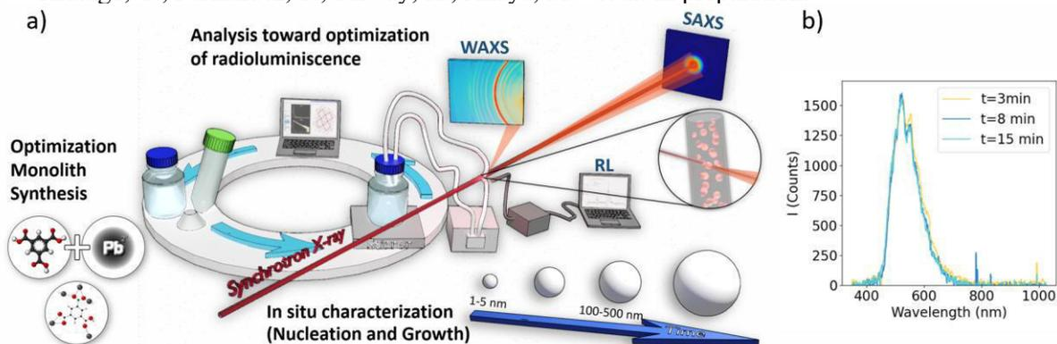
**Figure 1:** a) Process and setup for the in-situ flow experiment; b) Radioluminescence according to reaction time
