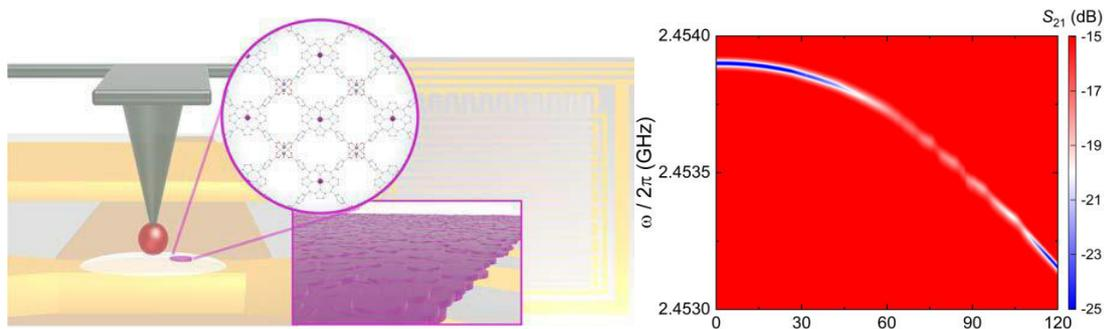
**Figure 1:** Scheme of in-situ formation of isolated nanodomains of the  $[\text{VOTCPP}]\text{Zn}_2(\text{H}_2\text{O})_2$  2D MOF on an LC resonator (left) and color plot of the microwave transmission of a resonator coupled to 10 MOF 2D planes (right).
