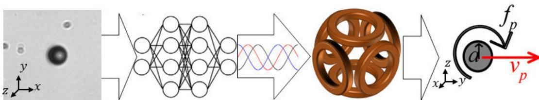
**Figure 1:** Schematic representation of the microrobot control process using deep reinforcement learning. From left to right: microscope image input, deep neural network for policy learning, rotating magnetic field actuation, and resulting roller motion.
