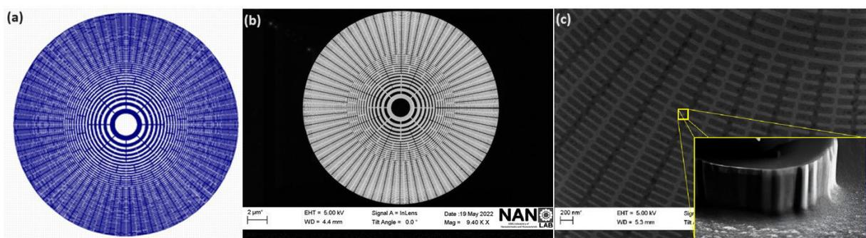
**Figure 1:** (a) CAD design of Fresnel zone lens, (b) Scanning electron microscope (SEM) image of FZP that has a diameter of 20  $\mu\text{m}$  and an outermost zone width of 50 nm, (c) SEM overview of FZP after 02mn of Silicone cryogenic -etching.
