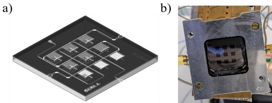
**Figure 1:** a) Design 3D schematics of the 3-by-3 LEKID array prototype camera. b) Picture of the prototype camera mounted in the measurement holder in the dilution refrigerator prior to RF characterization.
