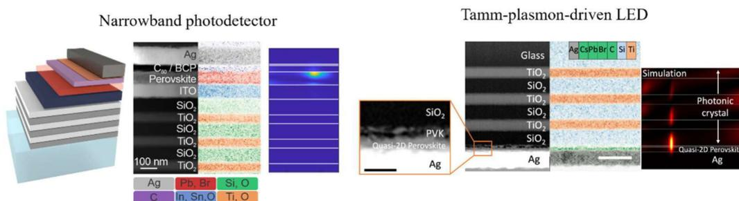
**Figure 1:** Scheme of halide perovskite optoelectronic devices: narrowband perovskite and tamm-plasmon-driven LED.
