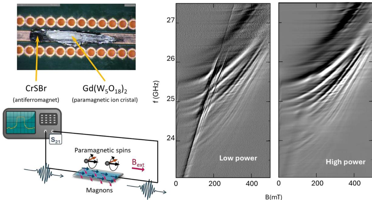
**Figure 1:** (Top left) Picture of the samples measured. Both materials lie on top of a coplanar waveguide connected to a VNA. (Bottom left) Scheme of the measurement setup. (Right) Derivative of the transmission coefficient  $S_{21}$  in two measurements at different power, where white (black) indicates positive (negative) value.
