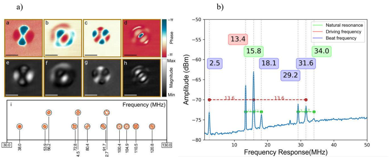
**Figure 1:** a) High resolution imaging of vibrational modes at 5 K. b) Spectrum analyzer response of an electrically forced resonator (driving frequency) and the lower and upper sidebands.
