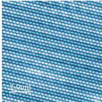
**Figure 1:** Intrinsic stripe order in 4H<sub>a</sub>-NbSe<sub>2</sub>
