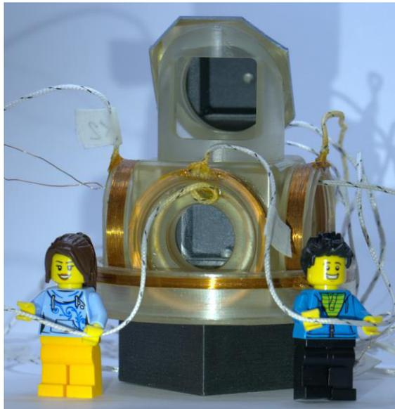
**Figure 1:** Levitation system and Pb levitating sphere
