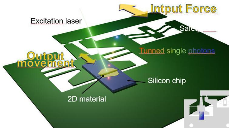
**Figure 1.-** A novel customized hybrid 3D-printed compliant mechanism device to introduce large strain fields in nanomaterials [1].
