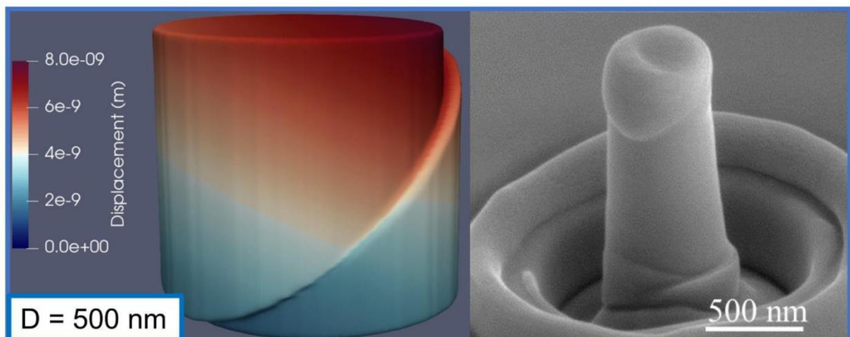
**Figure 1:** Residual deformation patterns for a 500 nm diameter W pillar [1] compared to SEM experimental observations [3].
