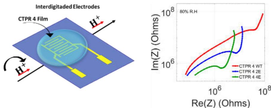
**Figure 1:** a) Schematic representation of a CTPR4 film deposited on interdigitated electrodes for electrical impedance spectroscopy characterization. b) Nyquist plots from EIS measurements of CTPR4 films prepared from different variants (WT, 2E, and 4E) at 80% relative humidity.
