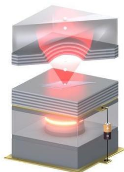
**Figure 1:** Schematic of the single photon device, composed by a quantum emitter in a hexagonal boron nitride monolayer, embedded in a reconfigurable Fabry-Pérot open cavity.
